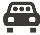
Car Traffic: 1-3 tonne (Load Class B for low speeds, D for Motorway speeds)
